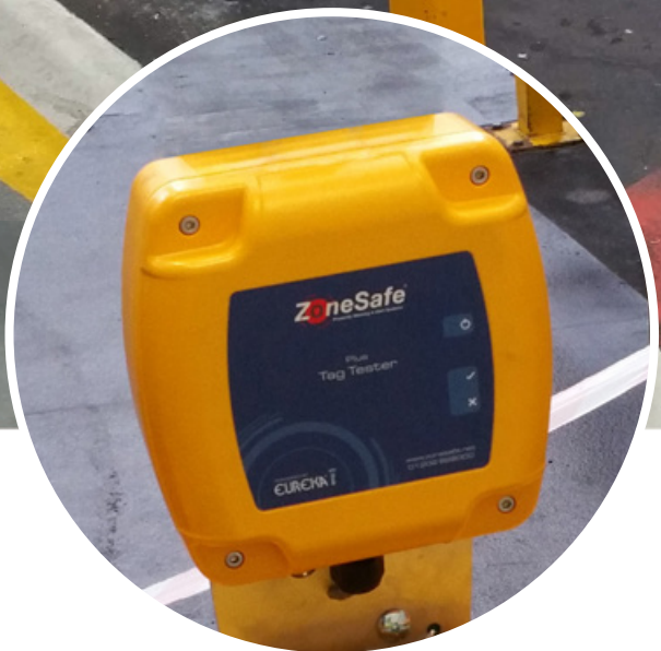
Tag Tester & Automated Gate Access
